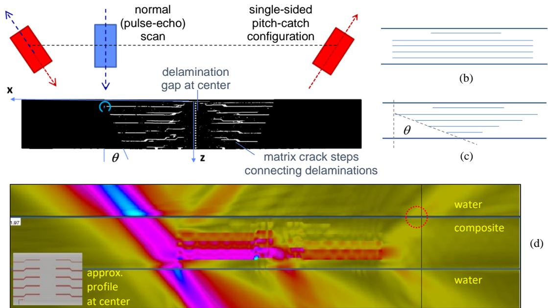
**Figure 1:** (a) Diagram of single-sided pitch-catch configuration for inspection of hidden delamination region of impact damage, showing micrograph of example cross-section. Diagrams of impact damage (b) columnar and (c) diamond profiles showing hidden damage angle. (d) Maximum ultrasonic response in 2D cross-section of columnar delamination profiles with insert showing approximate real impact damage profile at center of test sample.
