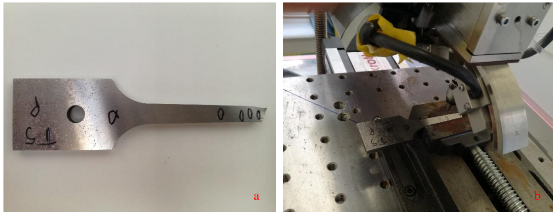
Figure. 1 a) The Inconel 718 specimen after fracture in fatigue test, and b) the same specimen during the X-ray diffraction experiment.
