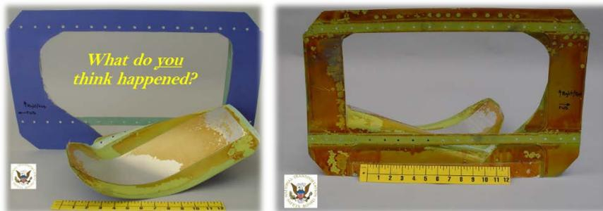
*Figure 1. Example of an in-service structural failure that is used for an inductive, team-based learning approach to fatigue cracking and the merits of fail-safe design [1].*
