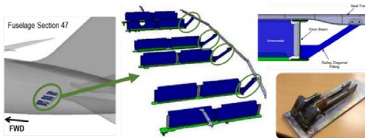
Figure 3. The certified 787 aft galley diagonal additively manufactured fitting.
