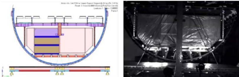
Figure 2. Fuselage drop simulation (left) and test (right) demonstrating 787 airframe crashworthiness.
