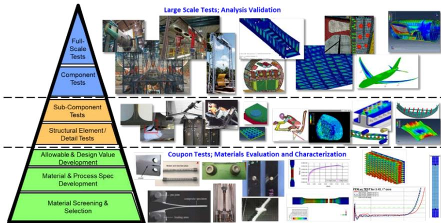
Figure 1. The structural test pyramid, with a smarter level of certification testing.
