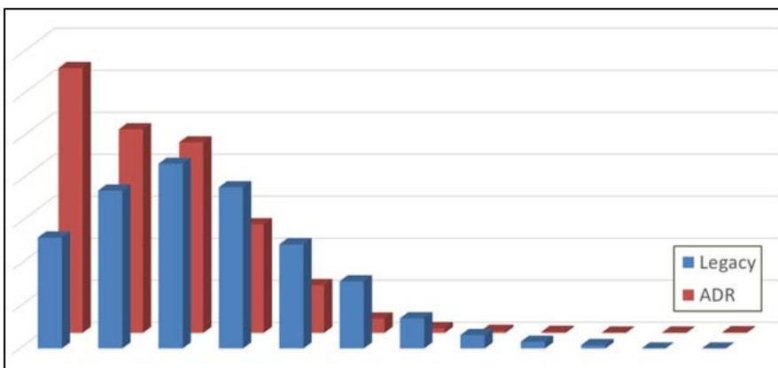
Figure 2. Histogram of landing sink rate design assumption (Legacy) and as recorded (ADR).
