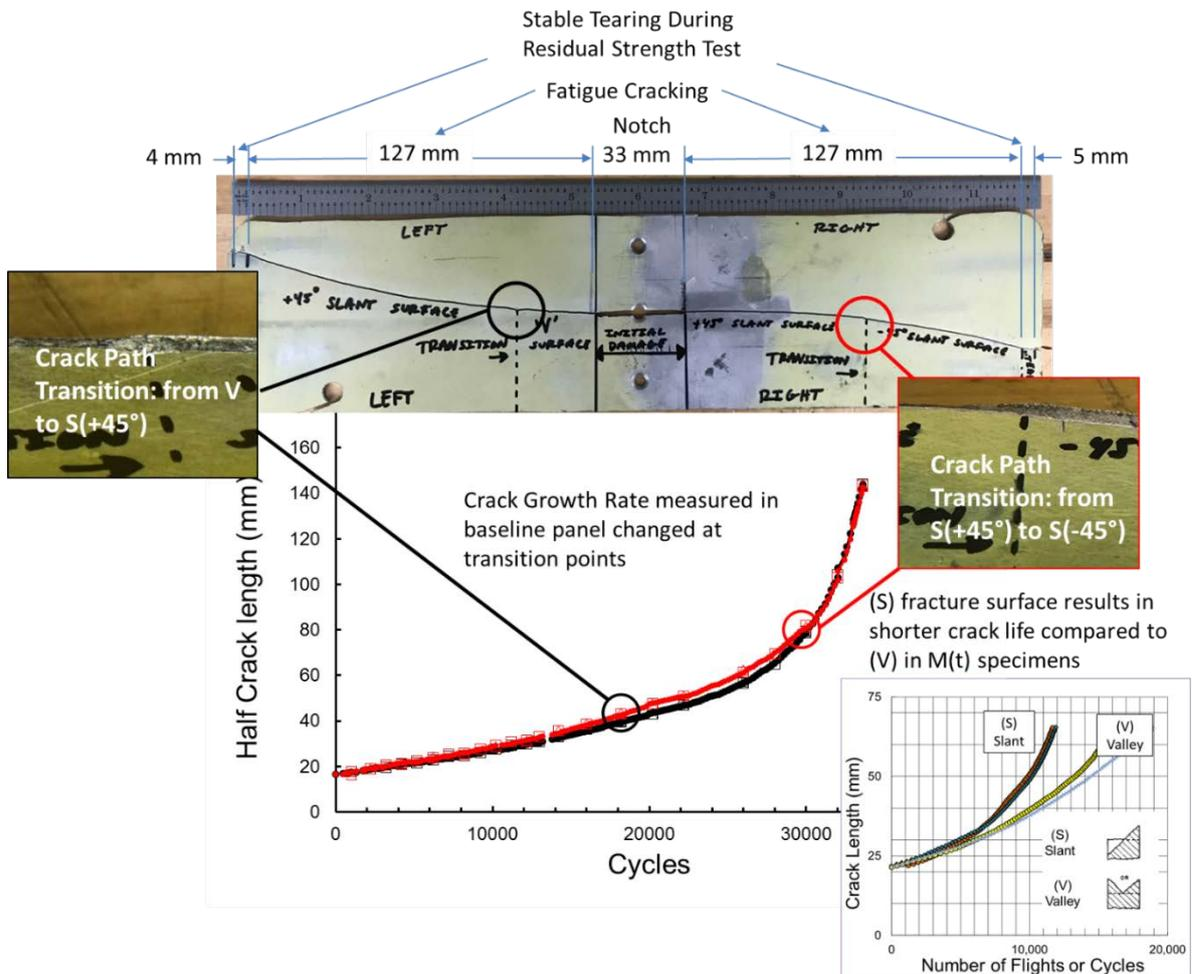
Figure 2: Phase I test results of baseline panel showing crack surface morphology and effect on fatigue crack growth.
