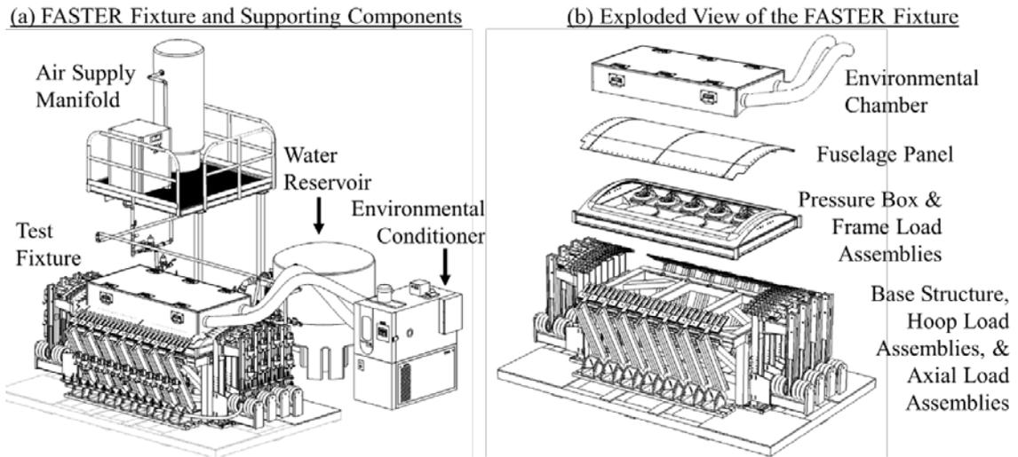
Figure 1. Full-Scale Aircraft Structural Test Evaluation & Research (FASTER) fixture
