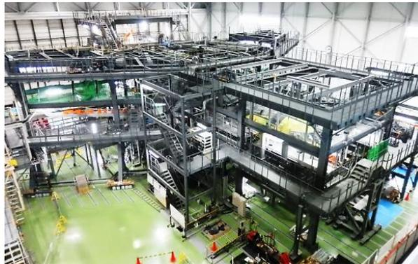
*Figure 1. MRJ full-scale fatigue test setup.*
