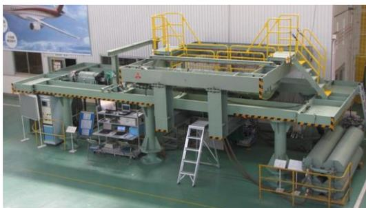
*Figure 2. Fuselage curved panel test setup.*
