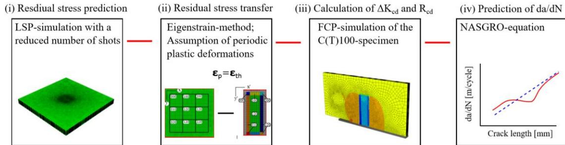
*Figure 1. Multi-step simulation approach.* The multi-step simulation takes the plasma-pressure as input and predicts the plastic deformations after the LSP-treatment (i). These plastic deformations are transferred to FCP-simulation based on the eigenstrain-method (ii). The FCP-simulation calculates the crack driving stress concentration factors (iii), which are used as input for the NASGRO equation (iv). Figure 1 is depicted and adopted from [1].
