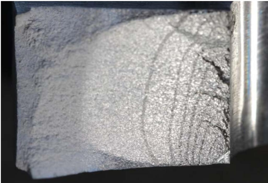
*Fig. 1 – Example of crack front evolution, from a mechanically milled notch.*
