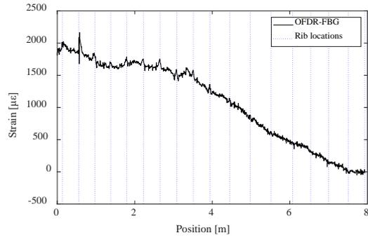
Figure 2. Strain distribution of main wing during banked turn..
