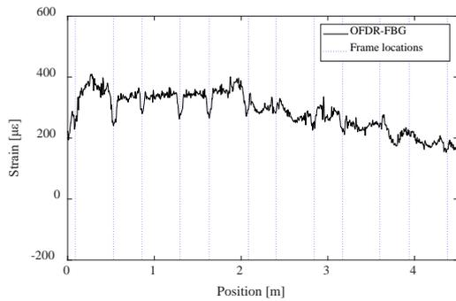
Figure 3. Strain distribution of fuselage stringer during banked turn..
