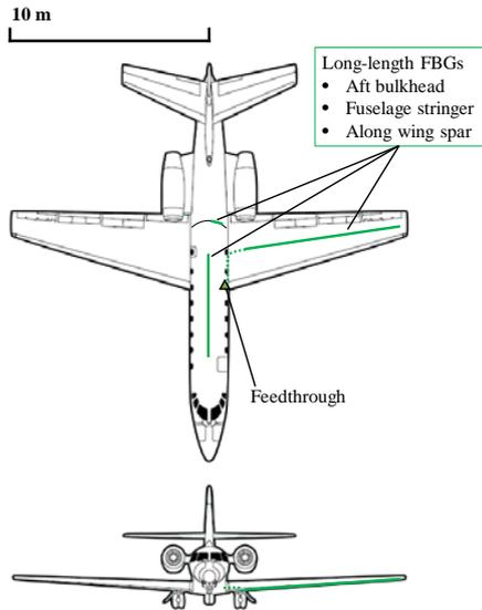
Figure 1. Sensing configurations for flight tests..
