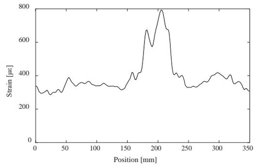
Figure 4. Strain distribution of aft-bulkhead after takeoff.
