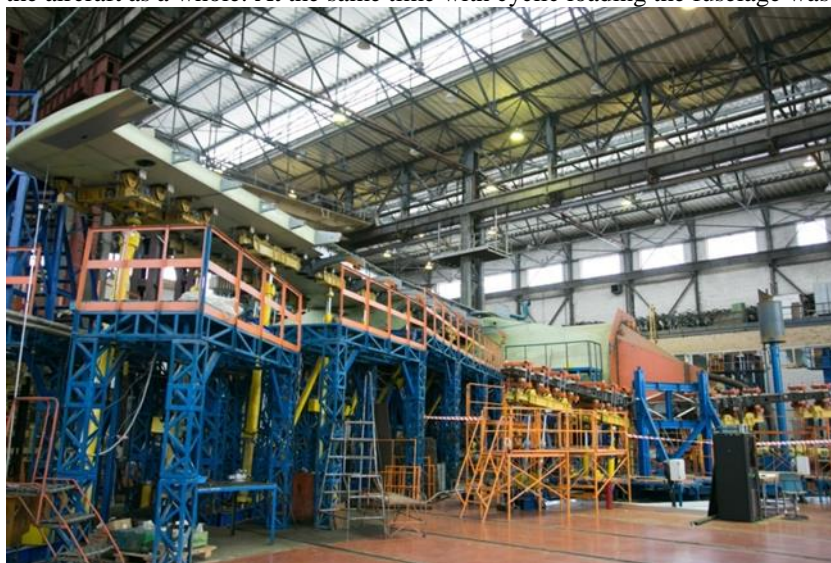
Figure 1. Full scale static-fatigue test set up.
