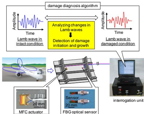
Figure 1. Overview of the ultrasonic based SHM system.
