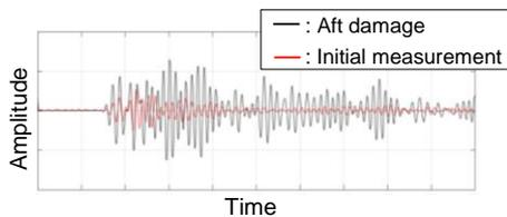
Figure 2. ultrasonic waves before and after damage measured in the test specimen.
